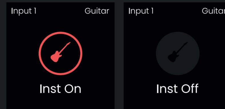
If you try and activate phantom power on Channels 1+2 whilst the instrument input is active, an error screen will show as it is not possible to have both active at once.
