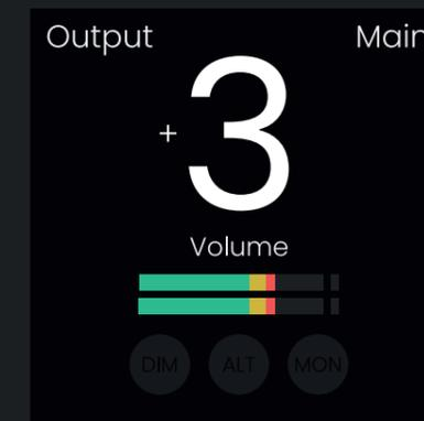
Whenever these features are toggled, the corresponding screen is displayed, before reverting back to the output status screen.
