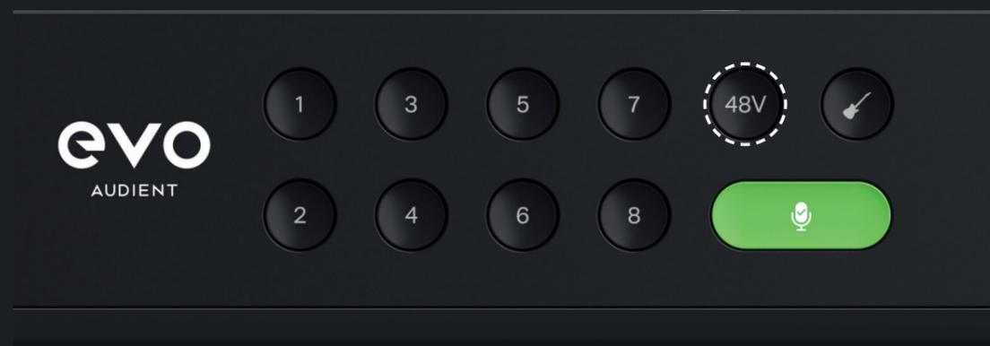
To activate phantom power, select the channel, then press the 48V button, which will then illuminate red as well as activate a temporary popup on screen.
