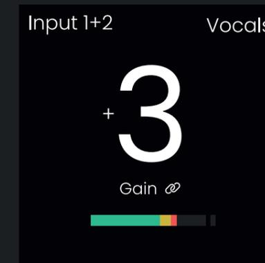
When on the input metering screen, you will also see a small hyphen connecting the linked channel numbers.
