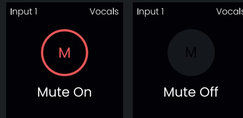
When a channel is muted, the gain level is replaced with the Mute icon, this will remain in place until mute is deactivated, by again holding down the channel button.
