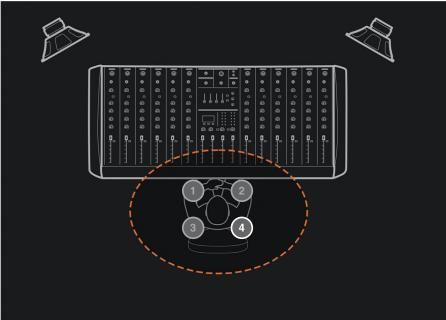
after 5 seconds the speaker will emit the calibration test signals (chirps).
