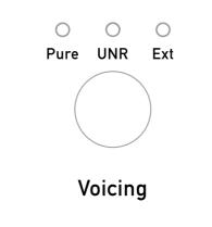
**Pure** is flat in anechoic conditions and offers the most linear, neutral, and highly accurate response that is suitable for mixing, mastering and critical listening applications.
