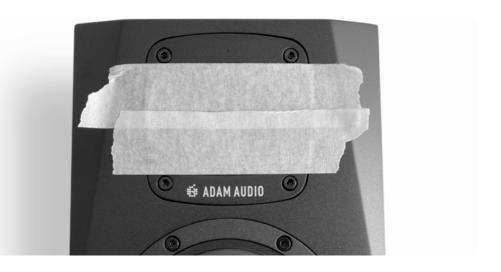
2. Using a standard hexagonal or "Allan" key, gently loosen all four screws on the front of the (5) waveguide.
