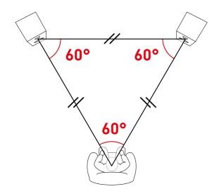
The A8H comes in two versions: left and right. Usually, they are positioned according (i) to the naming (left picture below), however if space is limited, for example in a very narrow room, it is OK to swap the loudspeakers (right picture below). When doing this ensure that the acoustic axis is still positioned with a 60° spacing so that the stereo imaging is unaffected.
