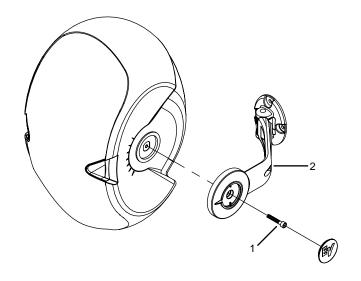
2. Attach EVID Speaker (1) to HS Series Stand (2) using the screw removed from step 1
