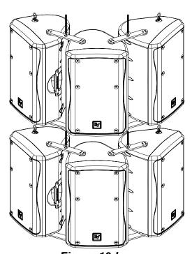
*Figure 10c:* Arraying Two Zx3's Two Enclosures High Using the Optional Array Bracket Kit
