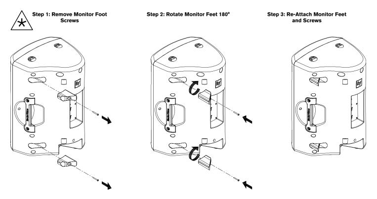
*Figure 11:* Switching the Monitor Feet from the 45° to 55° Positions
