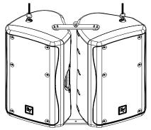
*Figure 10a:* Arraying Two Zx3's Using the Optional Array Bracket Kit
