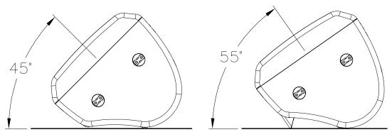
*Figure 12a: Zx*3 as Monitor in 45° Position
