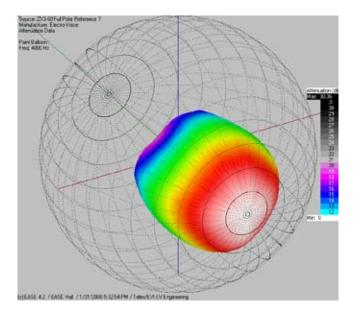
*Figure 1a:* 3D EASE Directivity Balloon, Zx3-60, 60° x 60° Coverage
