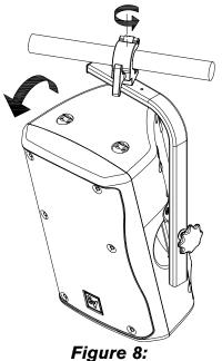
Suspending the Zx3 from a Truss Using the Optional Truss Mount Kit Kits Used -
