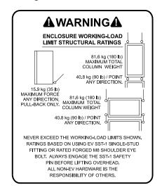
**Figure 2:** Working Load-Limit Rating of Zx3 Speaker System
