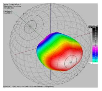
**Figure 1b:** 3D EASE Directivity Balloon, Zx3-90, 90° x 50° Coverage Electro-Voice® Zx3 Owner's Manual
