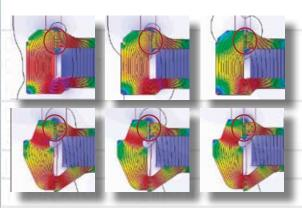
Snapshots of Dynamic FEA for a high power signal (100V) for a conventional design (top) versus DVX (bottom). The changing colors in the gap indicate an extreme variation of the magnetic flux for the conventional design, while there is only slight variation with DVX. The result is a more even travel of the DVX voice coil, significantly reducing harmonic distortion.
