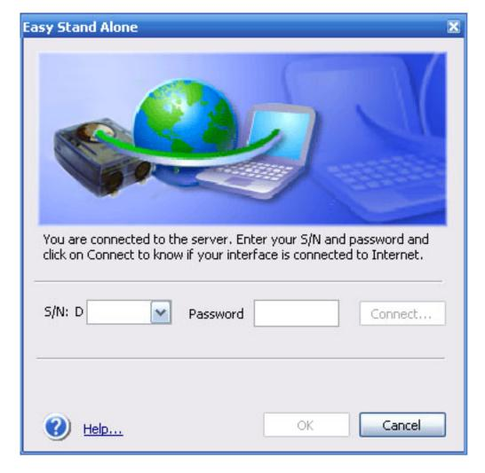
Here you must enter the S/N of your interface and the password and press connect. The default password is JULS. The software will tell you if the interface is connected to the Internet or not. If yes, you will be able to instantly upload the show and modify the interface settings. If not, you can upload the show to our server and the interface will download it as soon as it gets connected.
