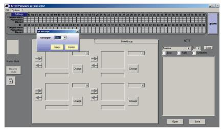
2.3 Click on System - Settings to configure which COM port use, the COM port of K-USB, usually is  $the \ higher \ number. \ If you don't find, you can \ check \ it on \ windows-control \ panel-system-hardware-COM \ Port$
