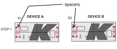
Unscrew the 4 anchor points of the front panels and remove it.
