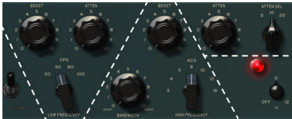
Control grouping within the Pultec EQP-1A
