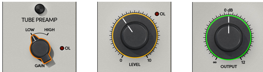
The three outlined gain controls as they appear when in Unison Gain Stage Mode
