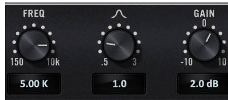
Bell Filter controls
