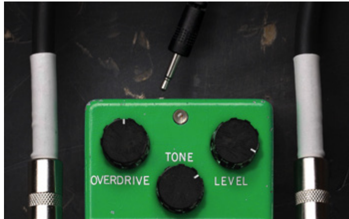
The unplugged power cable in true bypass mode
