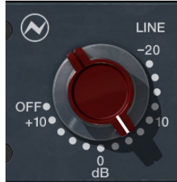
Line Gain control on 1073 Legacy plug-ins
