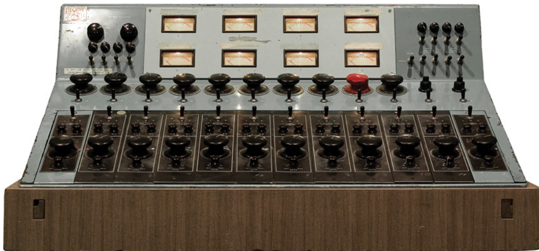
The original Wally Heider "Green Board" console containing 12 vintage UA 610-A preamplifier modules
